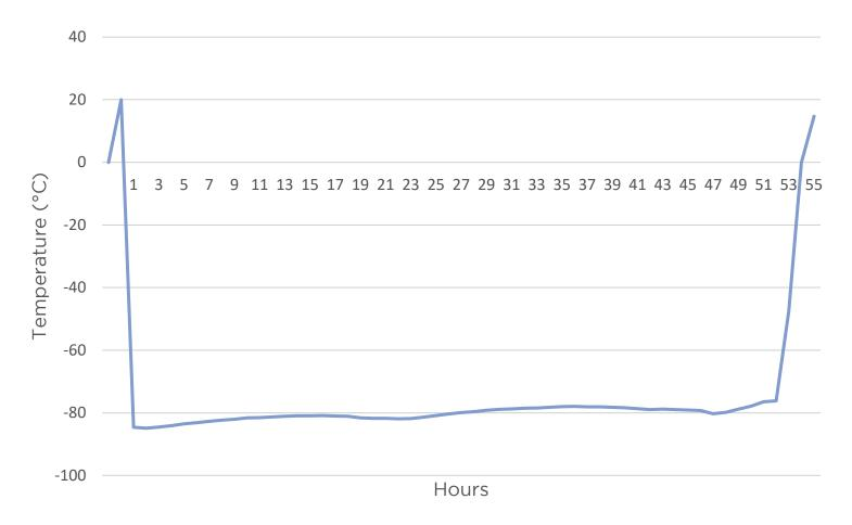
The test was carried out at an ambient temperature of approximately 19 degrees.
